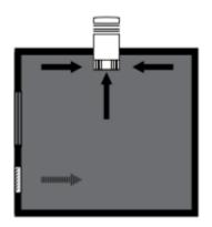
PVHR is a patented method of delivering high thermal efficiency and consistent air flow using natural ventilation systems by securely transferring the heat from exhaust air to fresh incoming air, in this case cooling it down. Supplying air through this method greatly reduced the problem in Oak Green, creating a comfortable learning environment.
